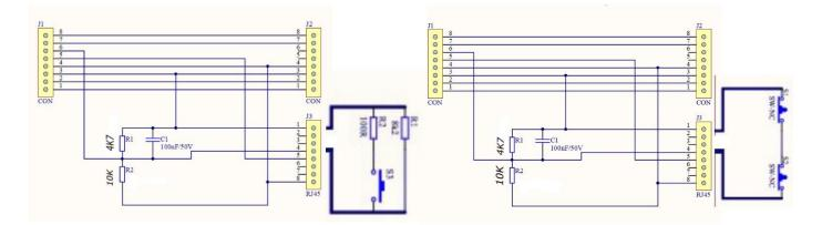
The picture shows the connection of a ribbon switch or sensing bumper to the safety input of the controller. The left side shows the content of the safety adapter, on the right side the part provided by the customer is shown in bolt lines. The 100 Ohm resistor represents the contact resistance of the ribbon switch.
